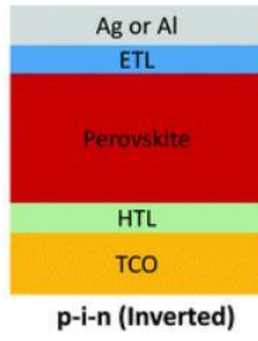
Figure 2. 8. Inverted Perovskite Solar Cell Device architecture [22]
