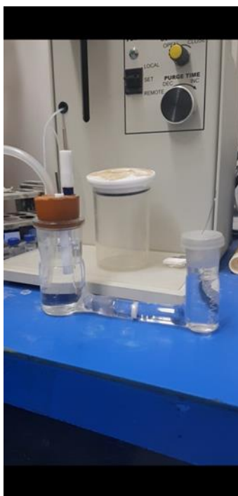
Fig 3.9 Schematic Illustration of an active H-type cell
