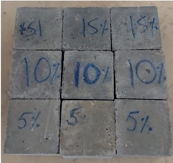
Figure 8. Cement composite samples with 5%, 10%, and 15% biochar content for compressive strength testing
