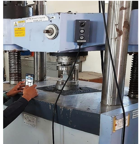
Figure 7. Cement composite sample in the Universal Testing Machine (UTM).
