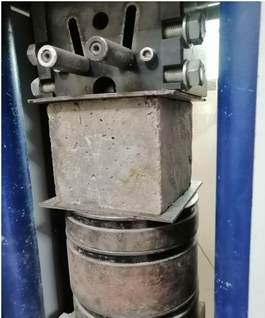
Figure 8 Compression testing apparatus
