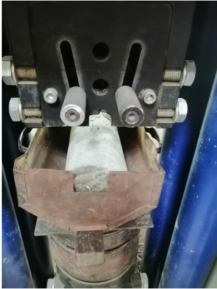
Figure 10 Cylinder Test (Split Tensile Test)
