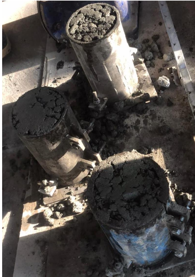
Figure 5 Cylinders during casting
