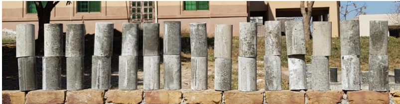
Figure 6: Cured NGW Cylinders (before being put in accelerated test setup)
