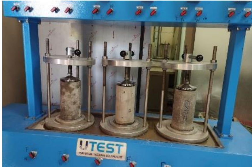
Figure 13: Samples Set in Apparatus for Permeability Test
