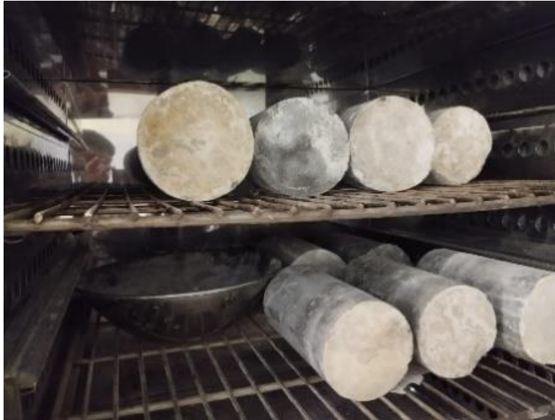
Figure 12: Samples Set to Dry for Water Absorption Test
