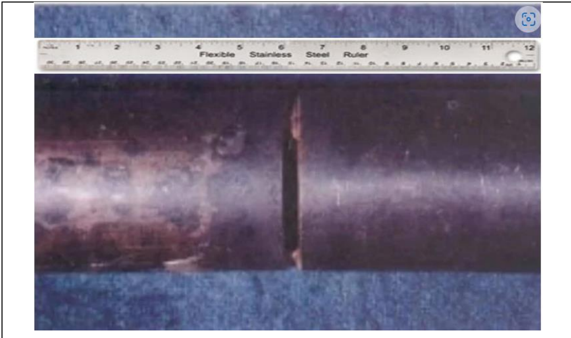
Figure 4. Vibration induced split.
