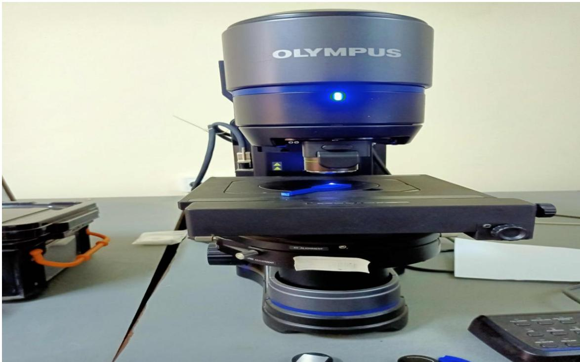
**Figure 2.5:** Olympus DSX 1000 Digital microscope
