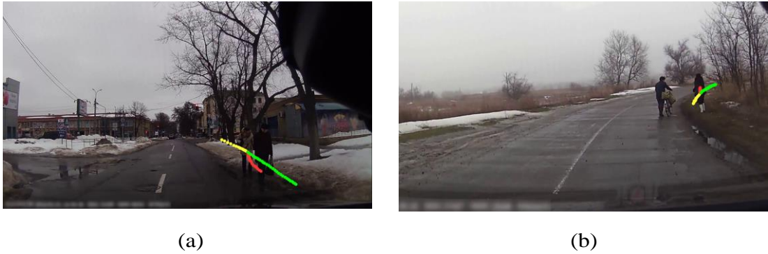
Figure 6.1: Failure cases. Yellow represents observed trajectory, Red represents the ground truth trajectory, Green represents predicted trajectory. (a) Failure because of lack of interaction information. (b) Failure because of lack of roads and lanes information.
