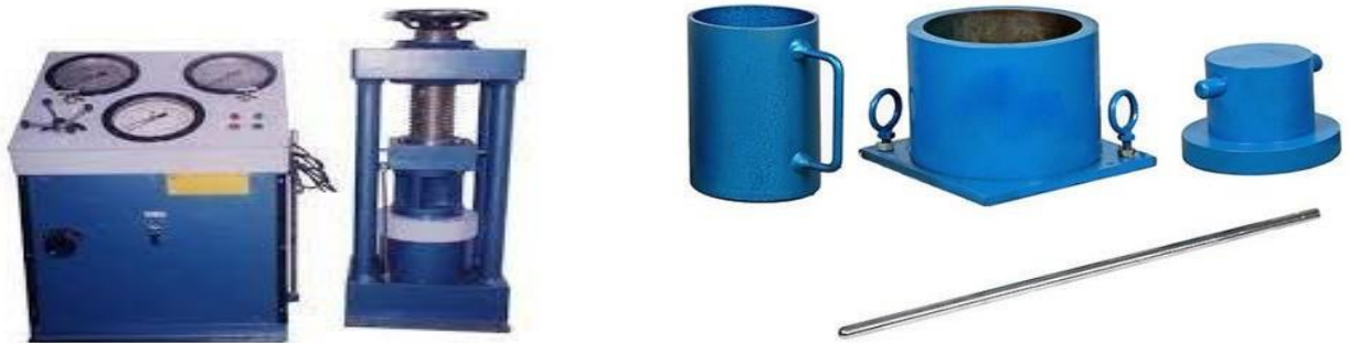
Figure 3-8 Crushing value test apparatus
