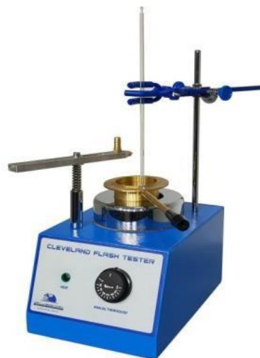
Figure 3-6 Flash and fire point test equipment
