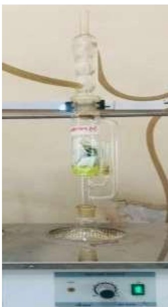
Figure 5 Ethanolic extract of Dodonaea viscosa prepared using Soxhlet apparatus
