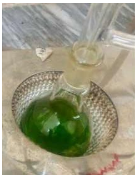
Figure 7 Ethanolic D.viscosa extract prepared using Soxhlet apparatus
