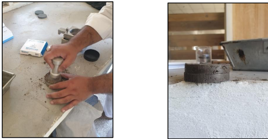
Figure 3.9: Preparation and failure of direct shear samples
