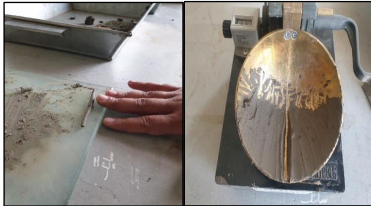
Figure 3.6: Liquid limit and plastic limit test
