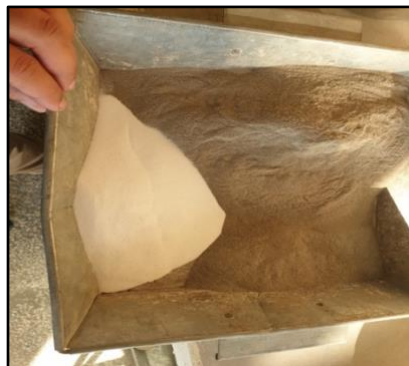
Figure 3.10: Soil, PET, and RCA for direct shear test
