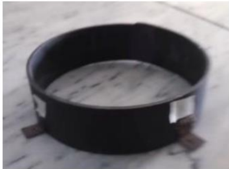
Figure 19: Steel Yoke employed for enclosing whole assembly.
