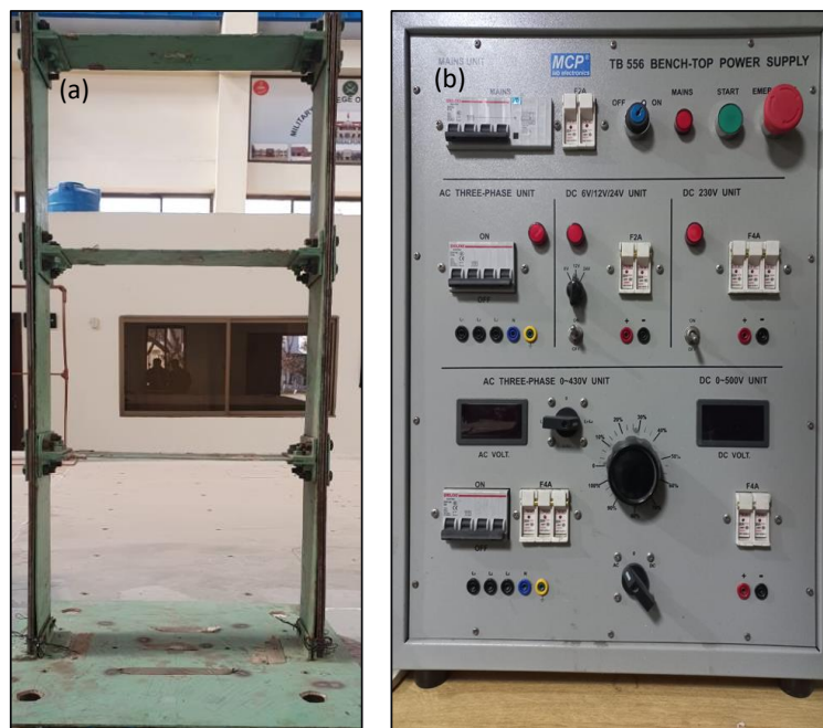
Figure 29: (a) Modified Steel Frame on Shake table (b) DC Supply for providing required values of current.
