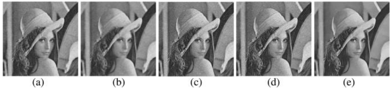
Figure 3.2: An illustration of image denoising [152]: (a) Wiener filtering [153], (b) Bilateral filtering [154], (c) PCA method [155], (d) Wavelet transform domain method [156], (e) BM3D [157].
