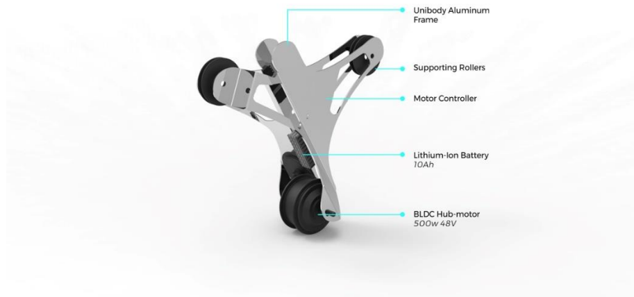
Figure 23. Final assembly of the wheel
