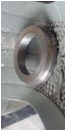
Figure w: press fit part for secondary nozzle
