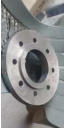
Figure t: flange for nozzle
