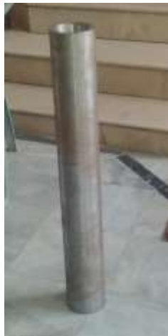
Figure y: internally tapered secondary nozzle
