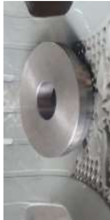
Figure x: press fit part for primary nozzle
