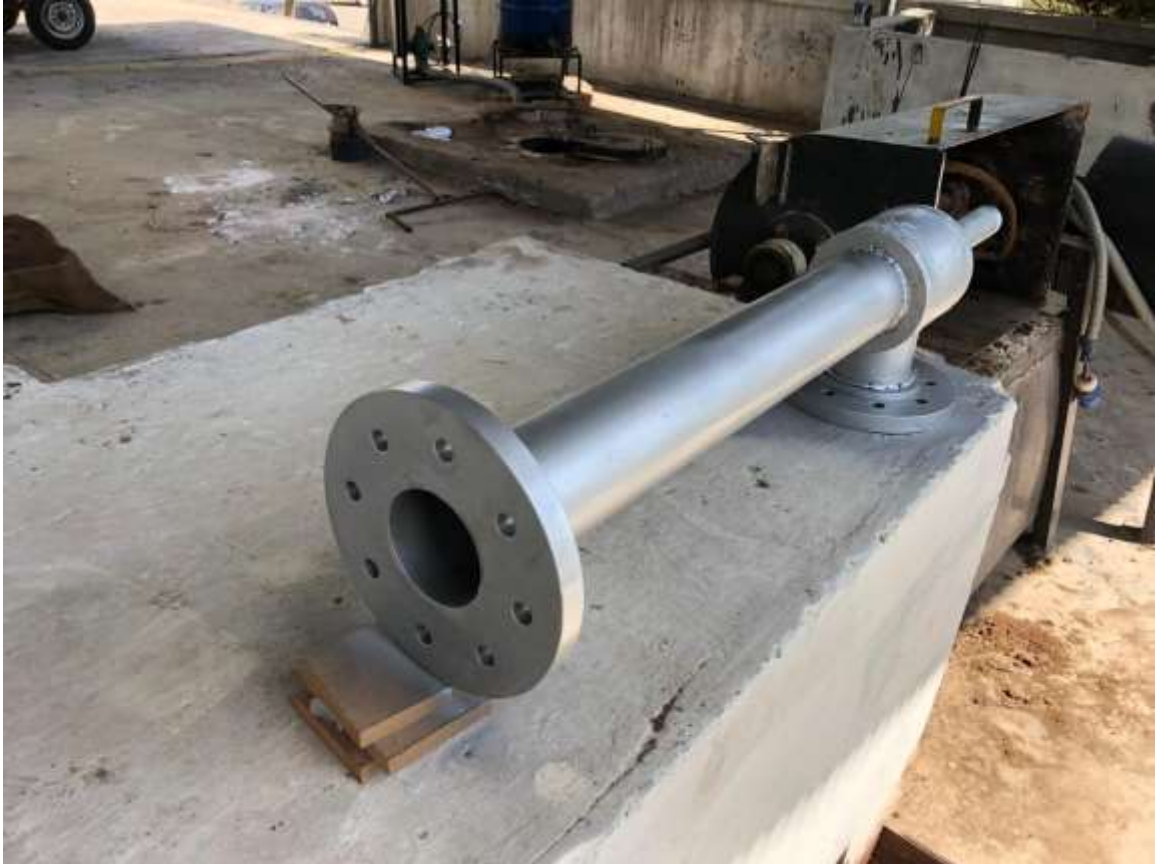
Figure z: ejector after being welded and painted
