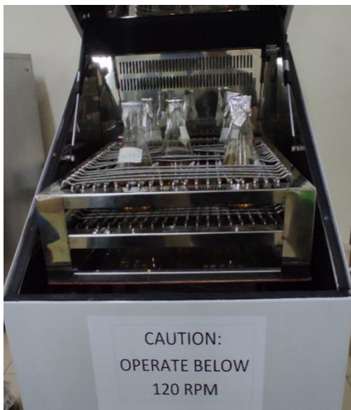
4. After inoculating the broth, the inoculum is kept in a shaking incubator for 48 hours
