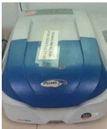
Fig 3.9 Spectrophotometer for obtaining OD 600
