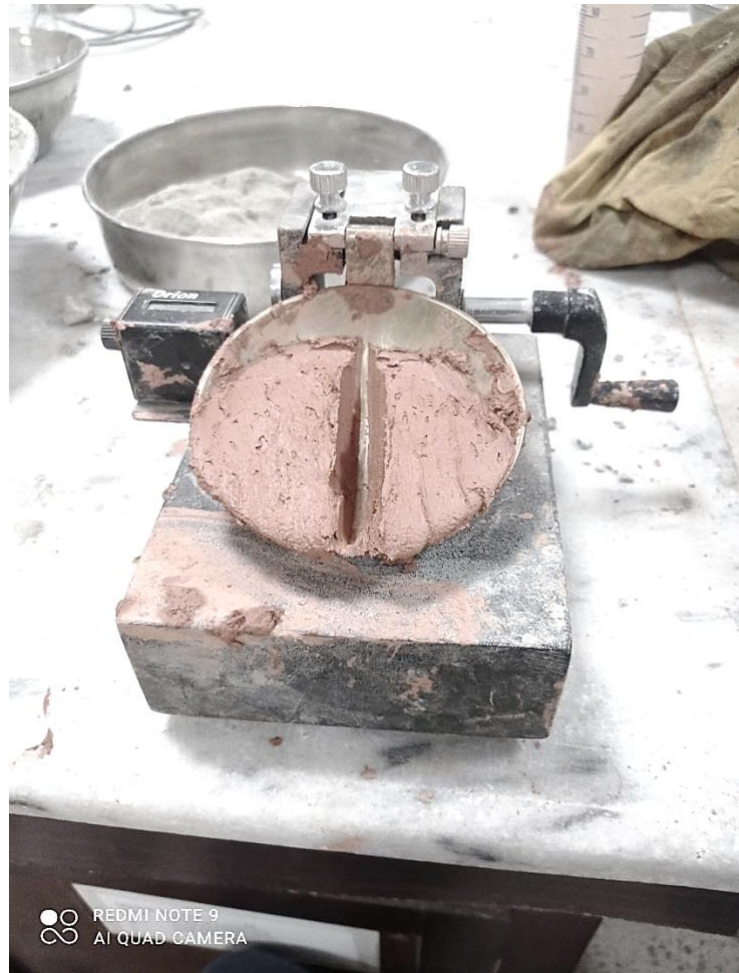
Figure 2.7 : Casagrande's Apparatus used for liquid limit
