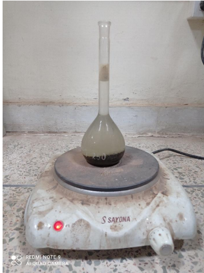
Figure 2.8: Pycnometer on a hot plate for conducting specific gravity test
