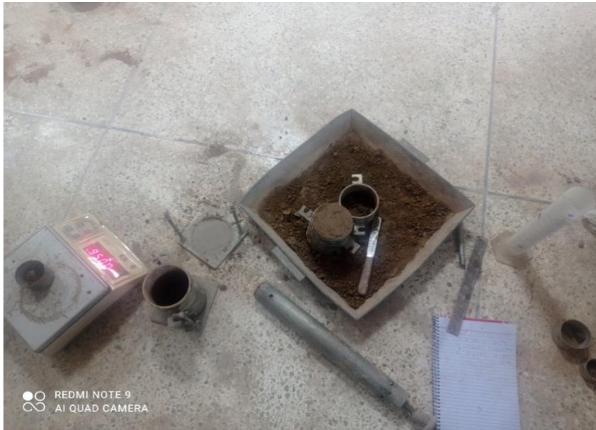
Figure 3.4: Apparatus for Standard proctor test in NICE Geotech lab
