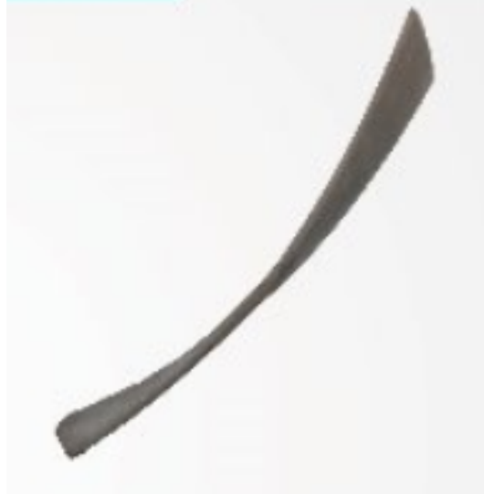
Figure 24-3D Printed Blade Pattern
