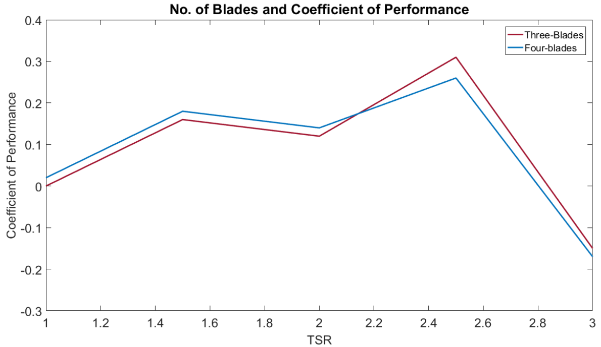
Figure 11-Effect of number of blades on turbine performance
