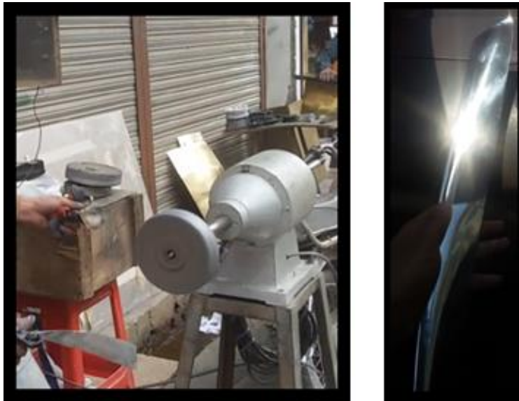
Figure 26-Grinding and Buffing of Blades
