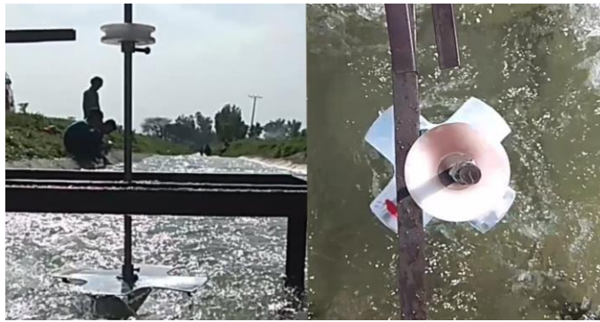
Figure 40-Turbine under operation (unloaded)
