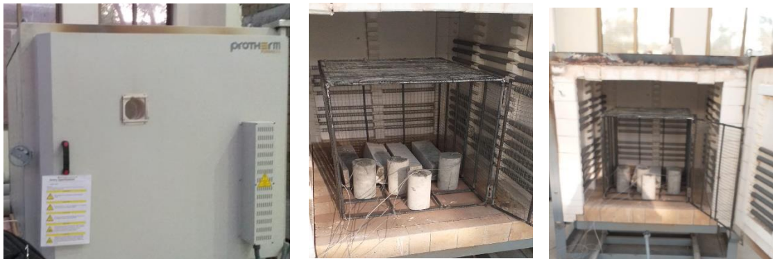
Figure 13 Electric furnace and Thermocouple attached with Samples
