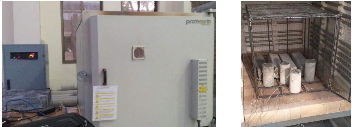
Figure 14 (a) Electric Furnace (range up to 1200°C) (b) thermocouples installed in samples for testing
