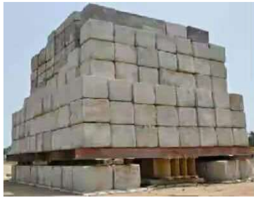
Figure 2: Pile Load Test
