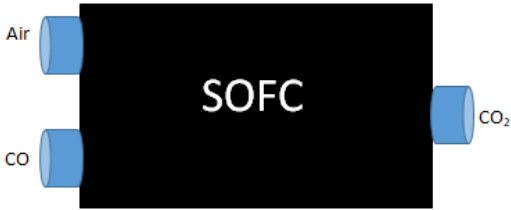
Figure 7. Basic sketch of a fuel cell showing the reactants and product of the reaction
