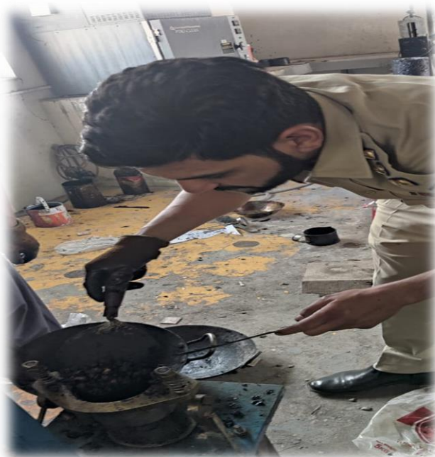
Figure 20 : Preparation of Semi Flexible Specimen
