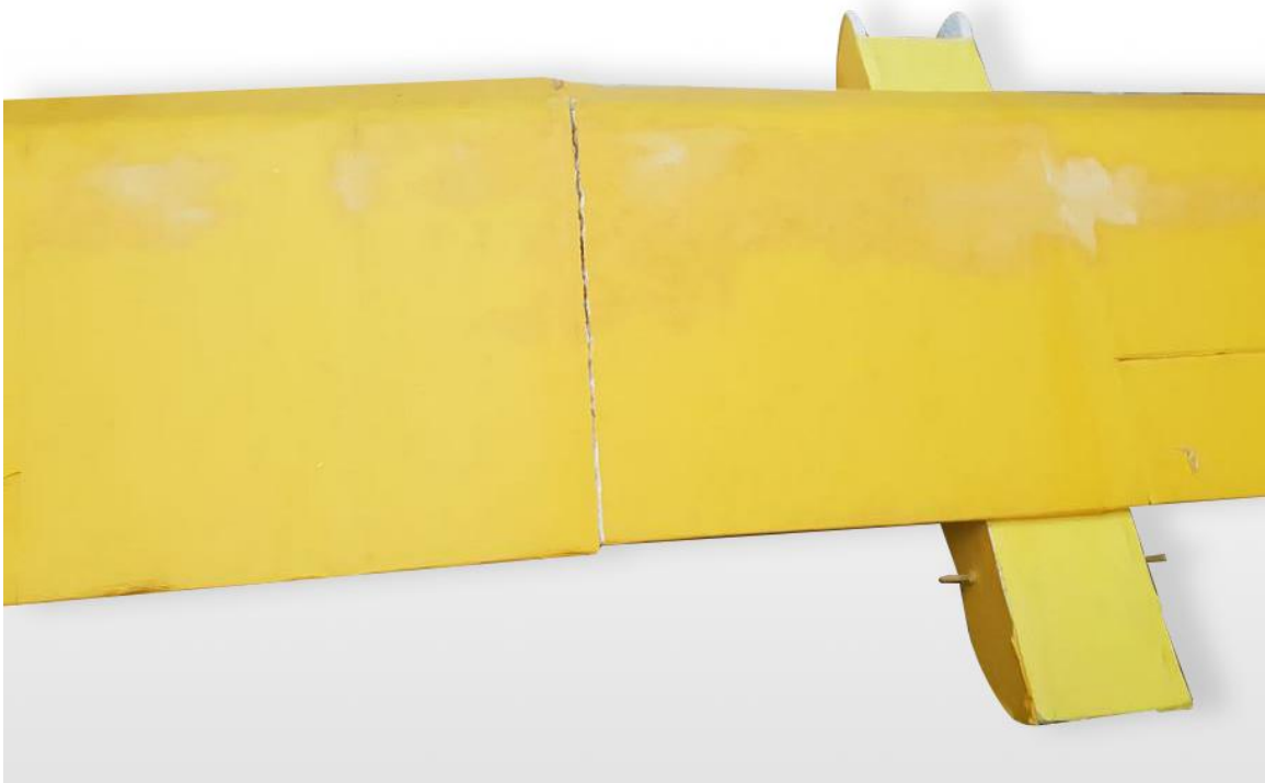
Figure 17 Damaged wing after the Second Flight
