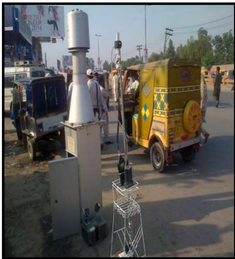
Figure 3.3: Sampling with High-volume sampler
