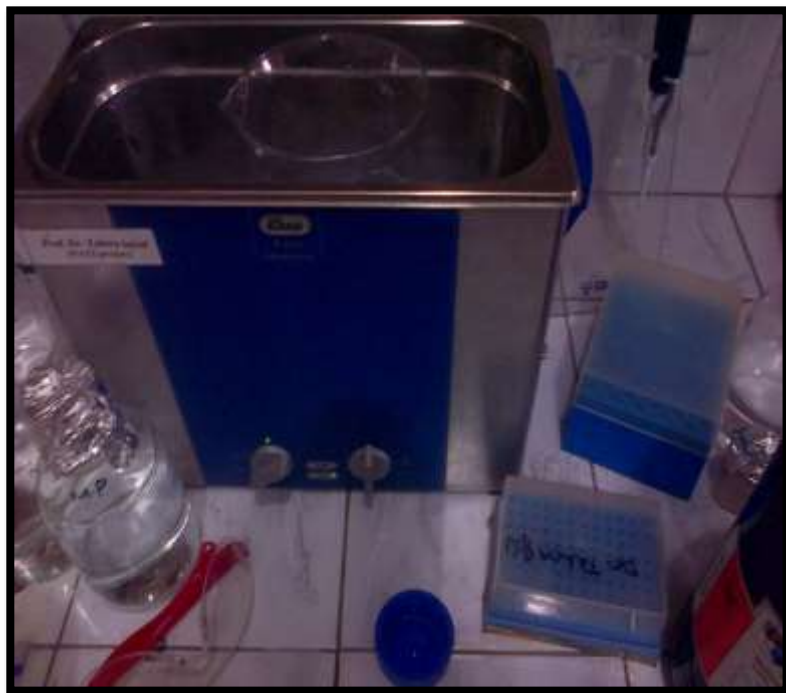
Figure 3.4: Sonication of sampled filters
