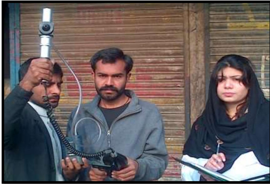
Figure 3.2: Sampling with Microdust Pro™ sampler
