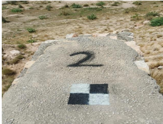
Figure 4 GCP no.2 having dimension 1ft x 1ft at the target site.
