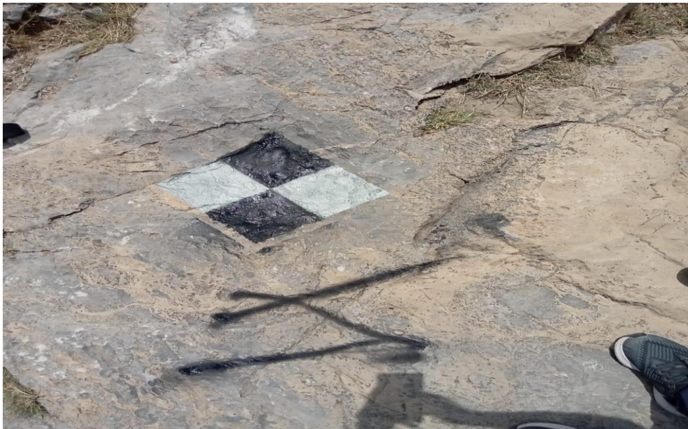
Figure 6 GCP number 4 is also the takeoff point for the UAV.
