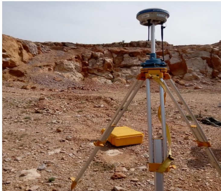
Figure 5 RTK Base Station placed at DHA Quetta
