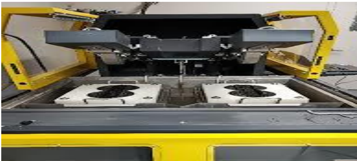
Figure 3.6: HWTT apparatus for rut depth calculation
