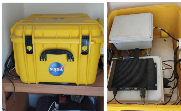
Figure 3.4: NASA Pandora Spectrometer main control box, containing spectrometer box, thermoelectric cooler, relay box, and computer.
