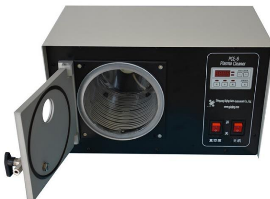
Figure 3.2. Plasma Cleaning setup
