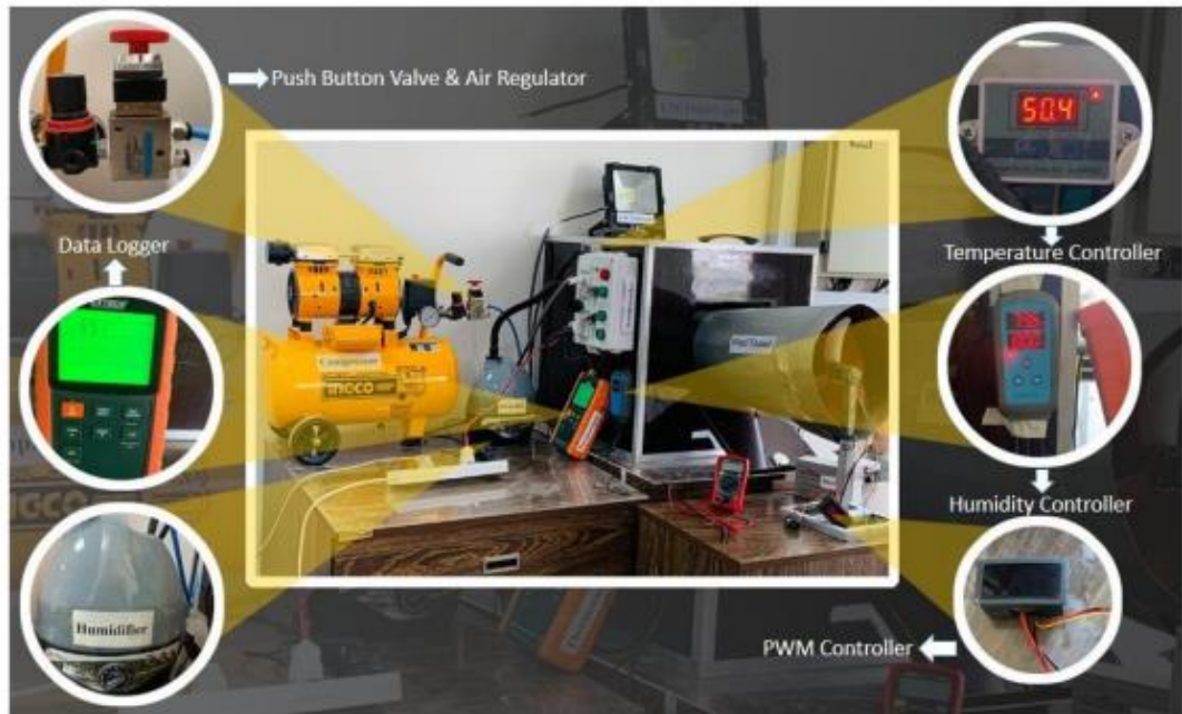
Figure 3.8. Setup of Indoor Soiling Chamber[13]
