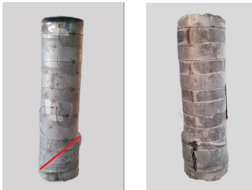
Figure 4. 18. Failure Mode of C1-Do/2
