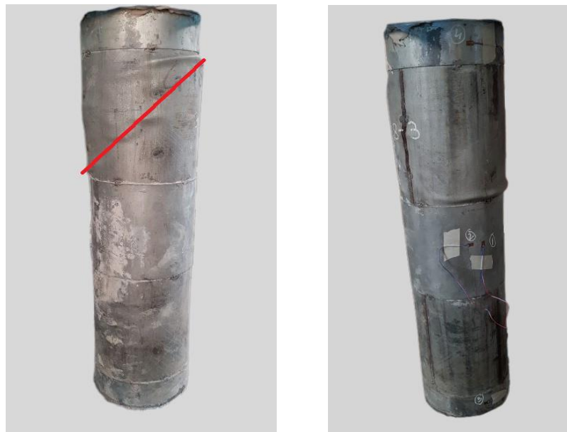
Figure 4. 9. Failure Mode of CFDST-4
