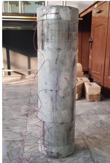
Figure 3. 9 CFDST Column with Strain Gauges
