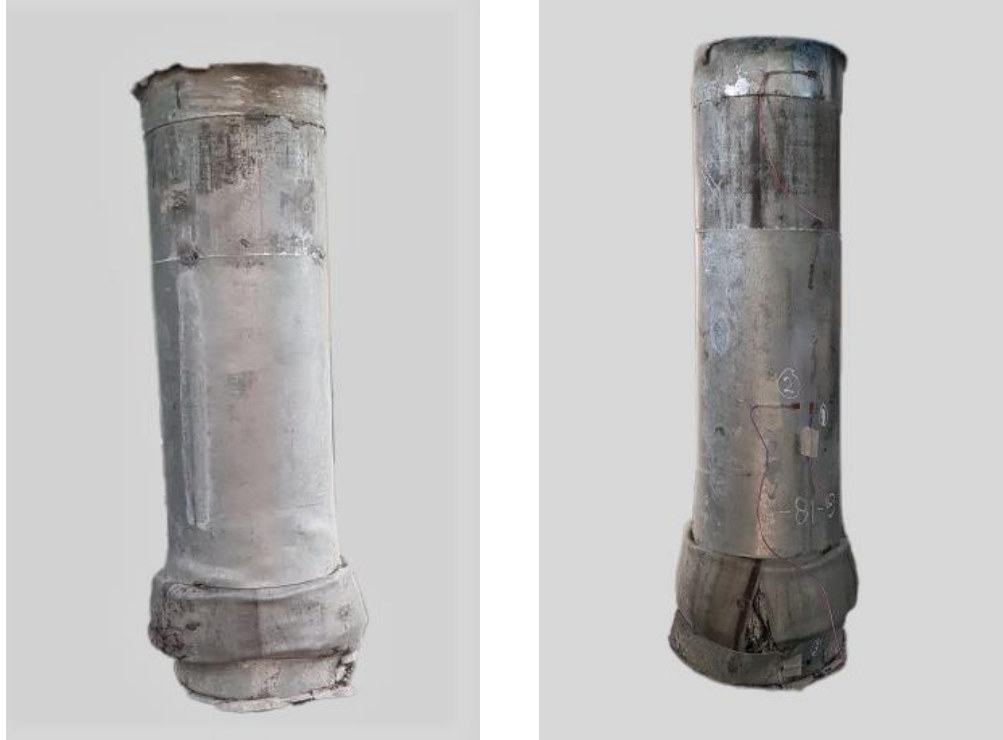
Figure 4. 15. Failure Mode of C1-2Do
