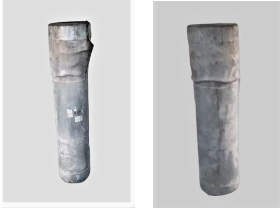
Figure 4. 12. Failure Mode of C1-1.5Do
