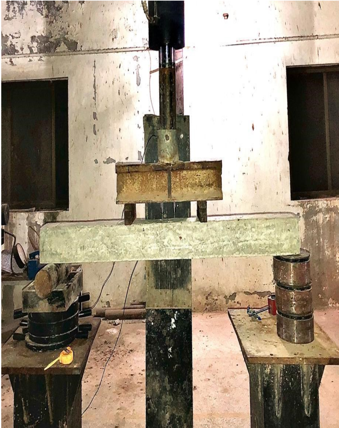
Figure 5 Experimental Arrangement of 4-point Flexural Test
