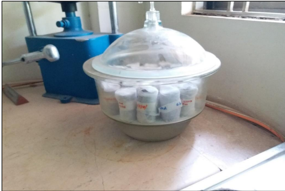
Figure 3.8: Soaking of UCS samples in a desiccator
