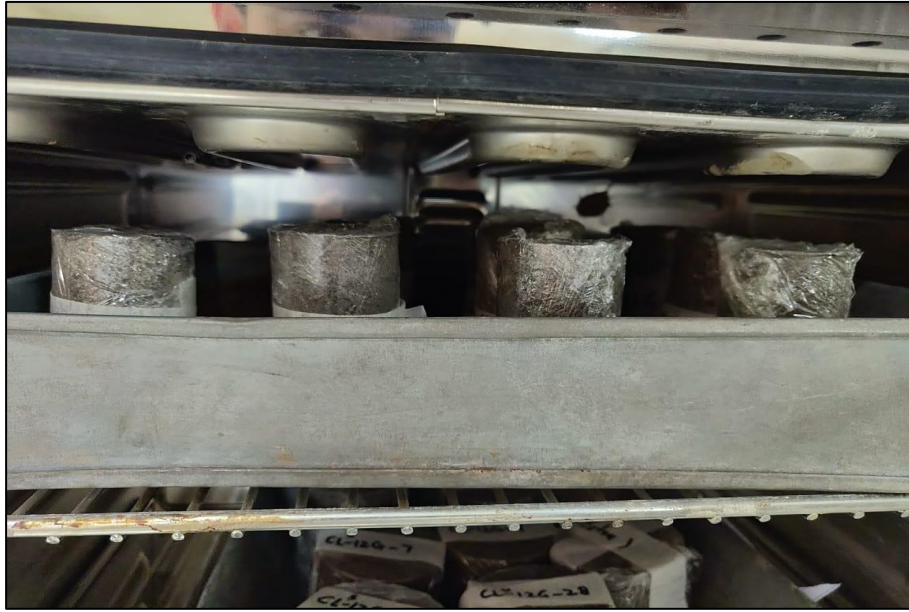
Figure 3.7: Curing of UCS samples in an oven
