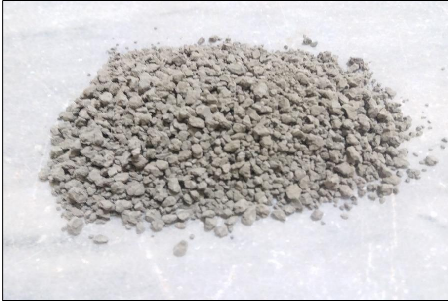
Figure 3.2: Soil sample passed through sieve #4
