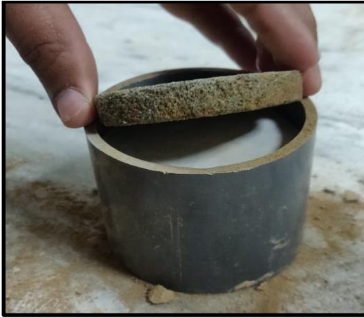
Figure 3.5: Sample preparation before applying wet and dry cycles
