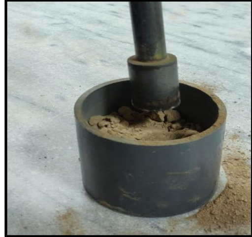
Figure 3.4: Sample compaction in the cylinders
