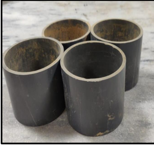
Figure 3.3: Hard PVC cylinders
