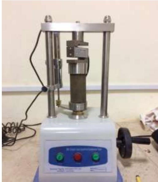
Figure 3.7: Sample testing arrangement in UCS apparatus
