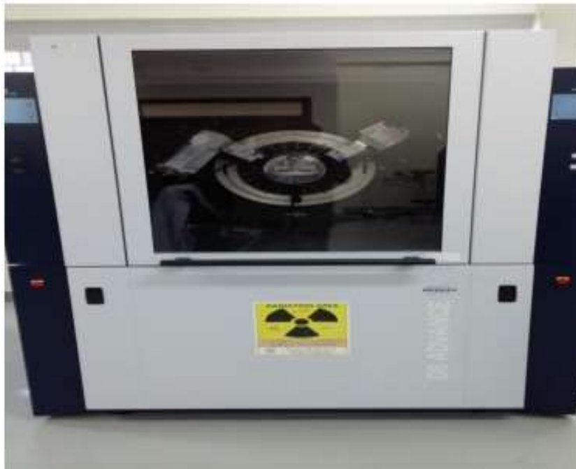
Figure 3.5: XRD apparatus (CASEN, NUST Islamabad)
