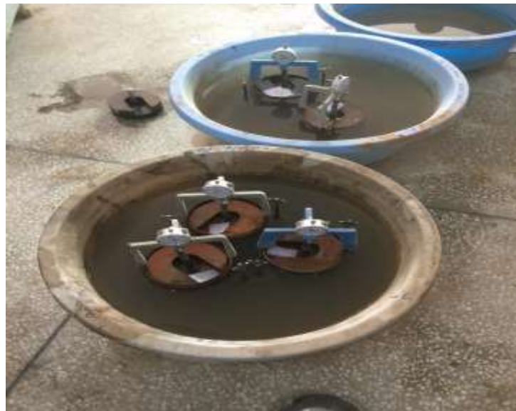
Figure 3.9: Soaking arrangement of samples for CBR test
