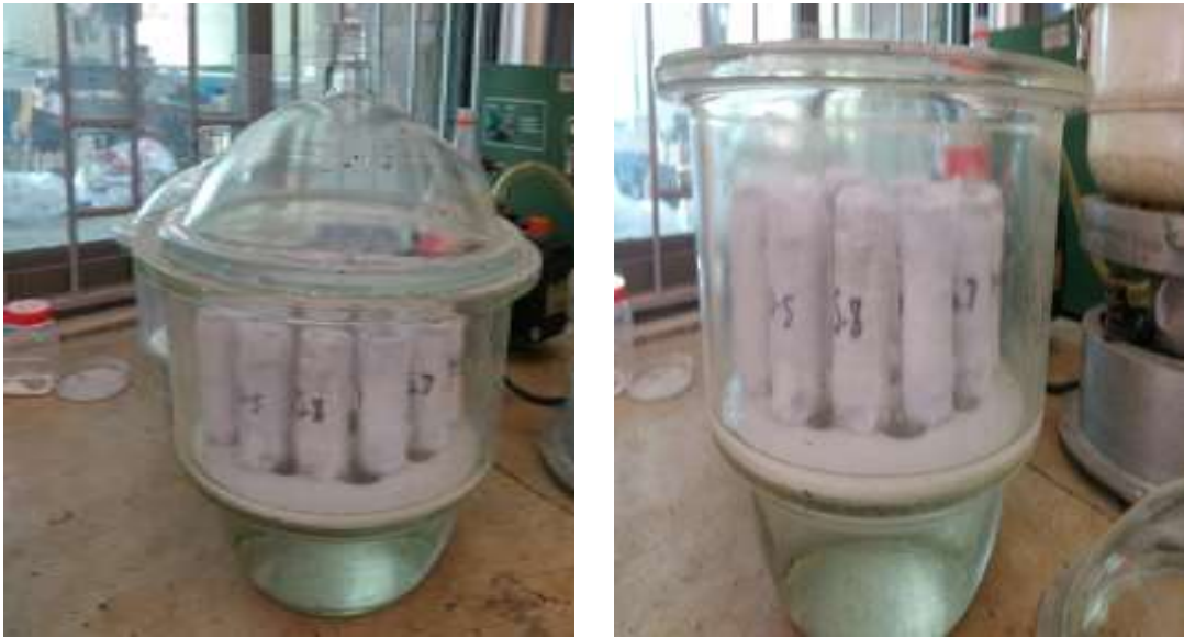
Figure 3.8 Soaked curing of samples for UCS test
