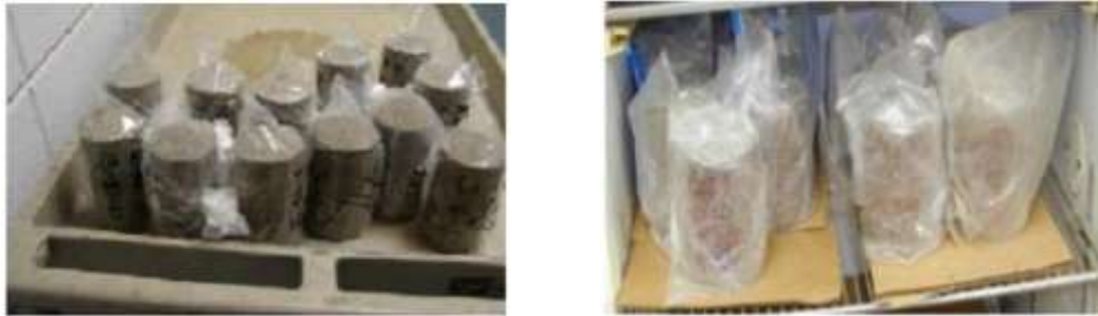
Figure 3.6 Un-soaked curing of samples for UCS test
