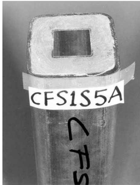
Figure 9 CFDSST stub column [10]
