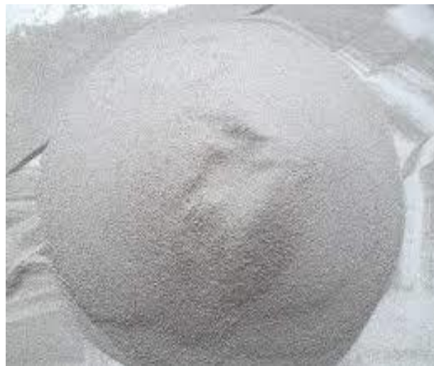
Figure 2.2: Fly ash cenosphere fillers
