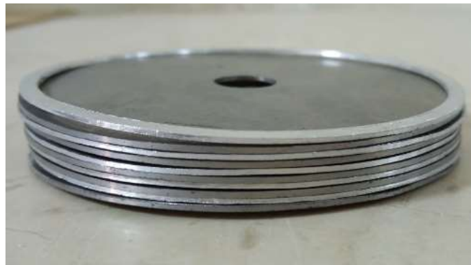
Figure 30: Steel Sheets and Aluminum Rings
