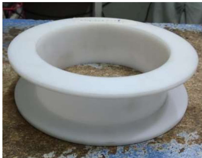
Figure 25: Non-magnetic Reel (148mm to 210mm dia, 5mm th.)
