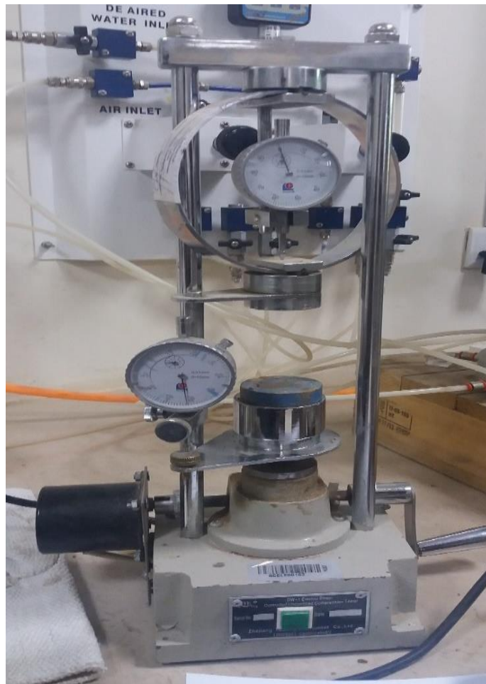
Figure 3.4: Unconfined Compression test apparatus
