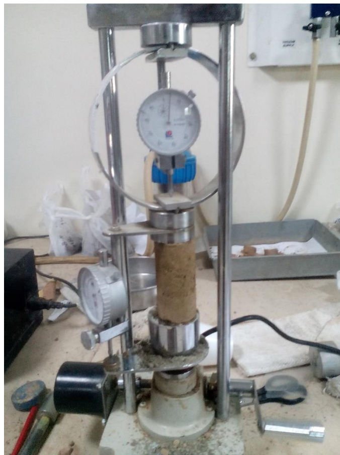
Figure 4.5: Unconfined compression testing
