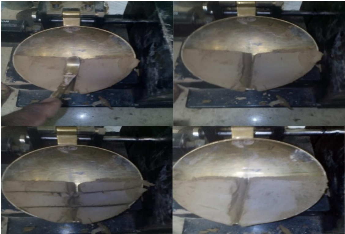
Figure 4.4: Determining Liquid Limit of soil samples by Casagrande's method
