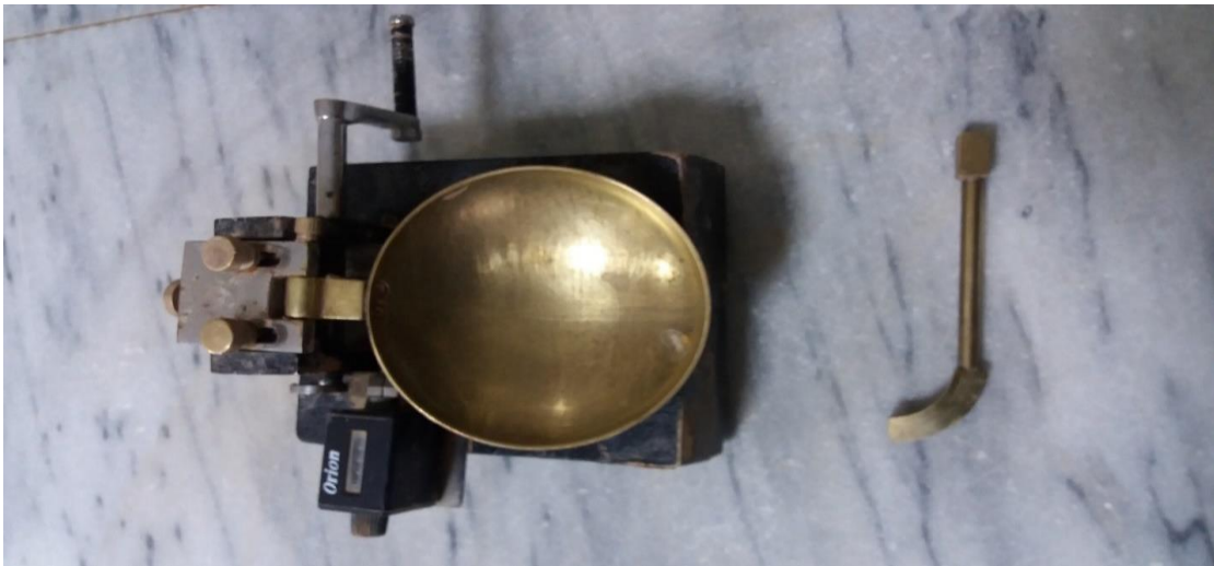
Figure 3.3: Casagrande apparatus with grooving tool
