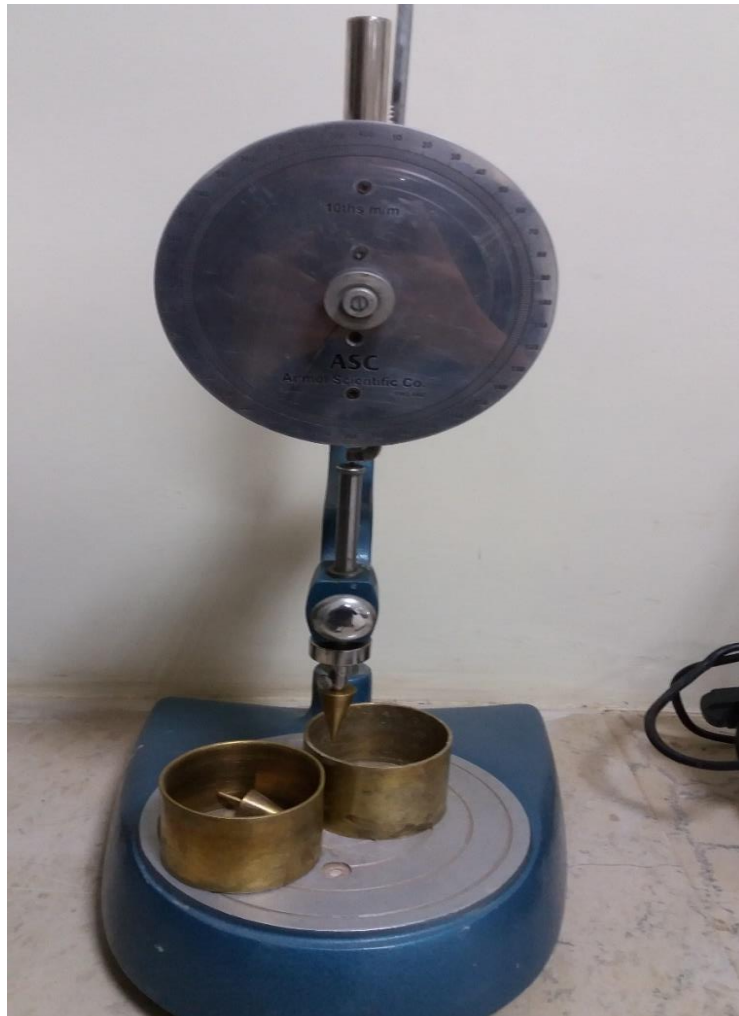
Figure 3.6: Fall Cone Penetrometer apparatus
