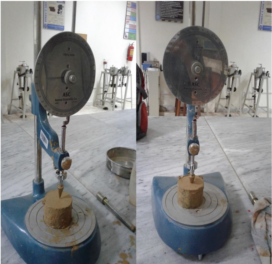
Figure 4.6: Fall Cone Penetrometer test
