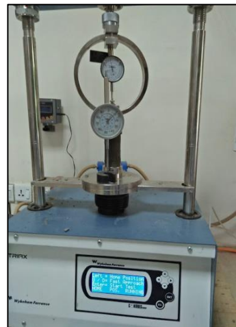
Figure 3.10: UCS sample testing
