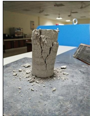
Figure 3.14: UCS failed sample
