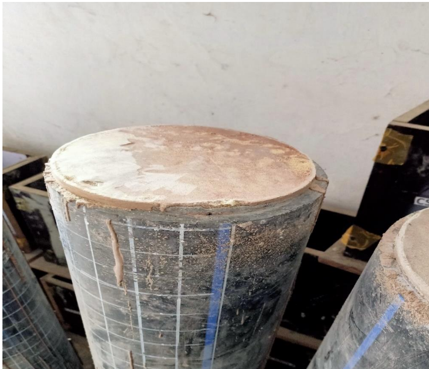
Figure 3.6 column capping with Sulphur
