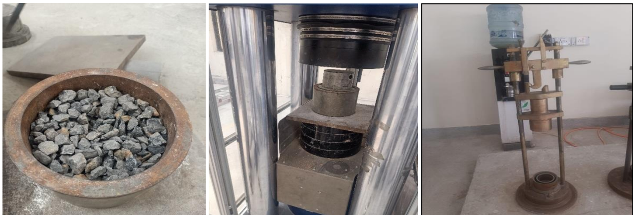
Figure 3.2 Impact value and crushing value test of Coarse Aggregate
