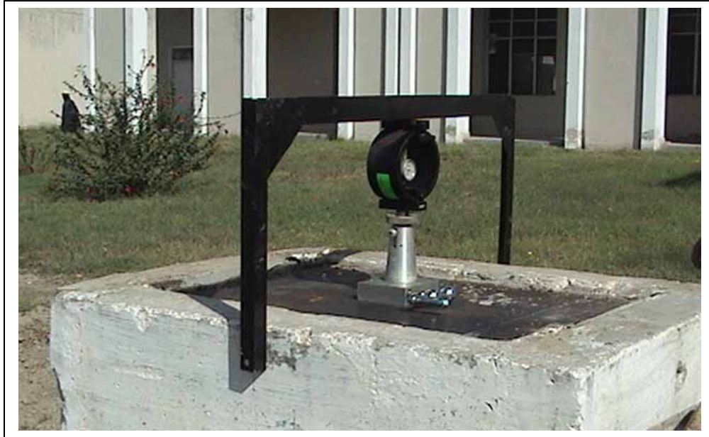
FIG. 4.7. Concrete Test Box and Jack Arrangement for Vertical Loading
