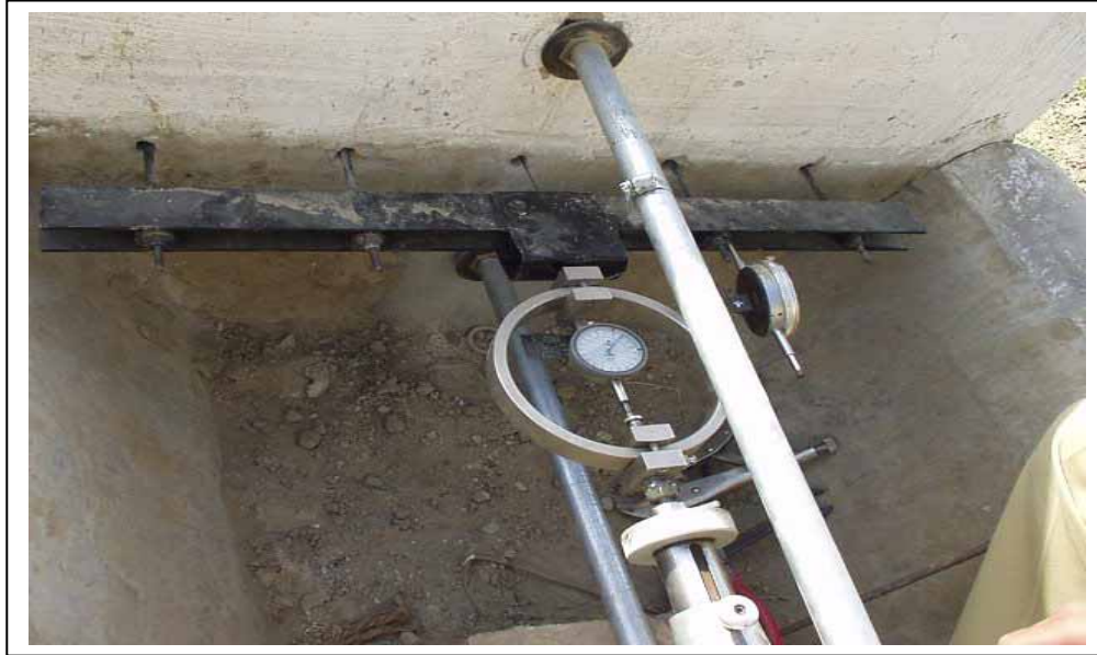
FIG. 4.6. Clamp, Proving Ring and Dial Gauges Arrangement
