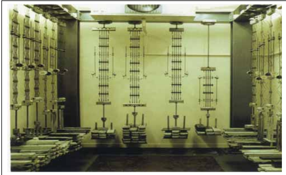
FIG.5.10. Pre-stretching Arrangement in Factory
