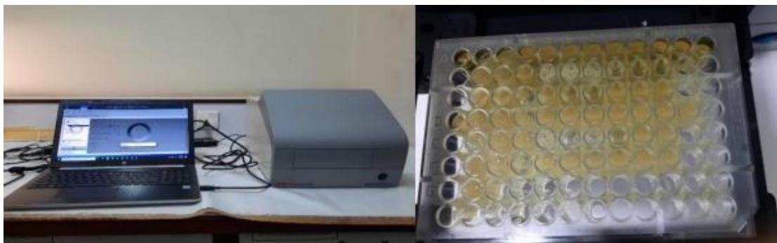
Figure 13 Microplate Reader in working and 96 well Flat Bottom Plate with Samples
