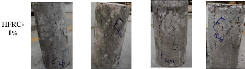
**Figure 16:** Compressive Failure Mode of Cylinders at Targeted Temperatures.
