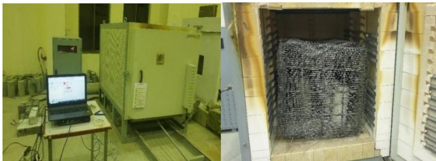
**Figure 8:** Electric Furnace for Heating the Samples to Targeted Temperatures.
