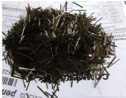
**Figure 1:** Chopped Basalt Fibers.
