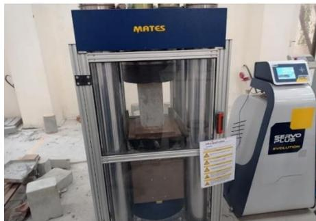
**Figure 9:** Compression Testing Machine.
