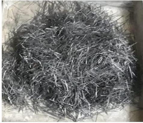
**Figure 2:** Steel Fibers.
