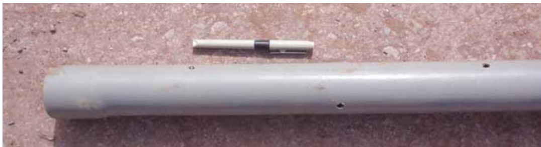
Fig. 3.7. Perforated PVC Pipe Used for Standpipe Piezometers.
