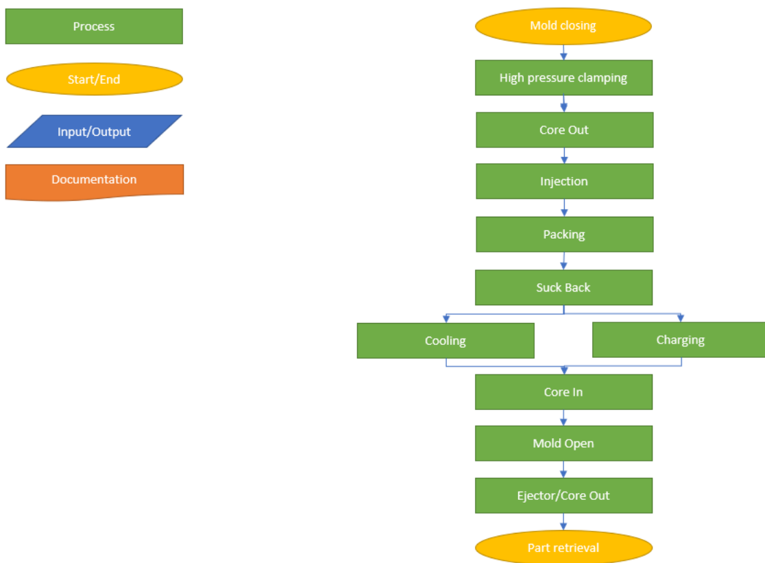
Figure 3.3 Process Flow for Injection Molding process
