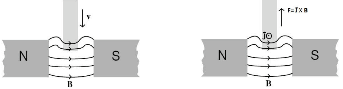
Figure 2.1: The two basic physical effects taking place in MHD. A moving conductor which modifies the magnetic field by dragging the field lines with it. In the case of infinite conductivity, the field lines look frozen into the moving conductor (Left). When electric current crosses magnetic field lines there will be a Lorentz force, which will cause acceleration in the fluid (Right).
