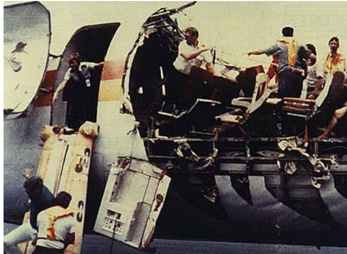
Figure 1: Corrosion Fatigue failure [5]
