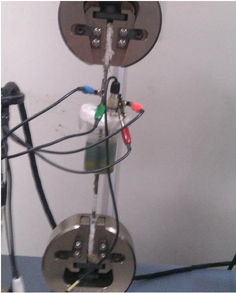
Figure 23: Cell Setup for Corrosion testing
