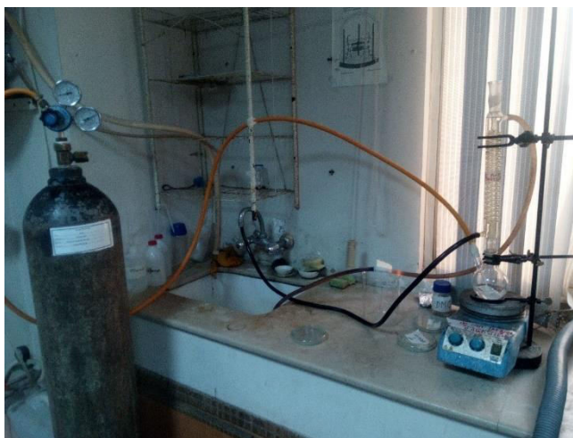
Figure 9 Initiator attachment on APTMS functionalized RO membrane
