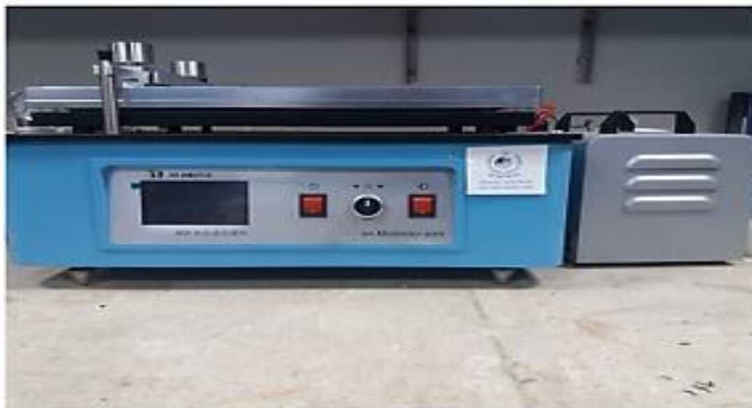
Figure 3. 1: Polymer membrane casting machine (Automatic Film Applicator, Elcometer4340 M43 6BU)
