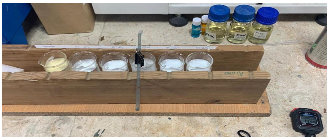
Figure 3. 4: Depicting the process of dip-coating formulated bi-layer coating
