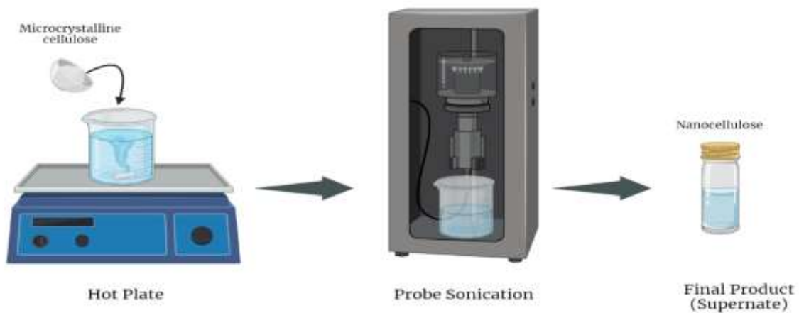
Figure 14: Synthesis of nanocellulose from microcrystalline cellulose through ultrasonication probe
